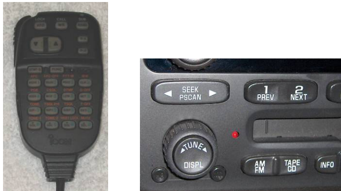
Figure 35 - Microphone for controlling a radio and the Tune knob on a car radio.
