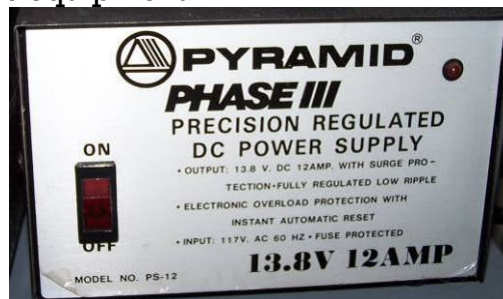
Figure 31 - Regulated DC Power supply. Photo by N5IUT
