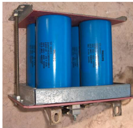
Figure 59 - Power Supply capacitors. Photo by N5IUT
