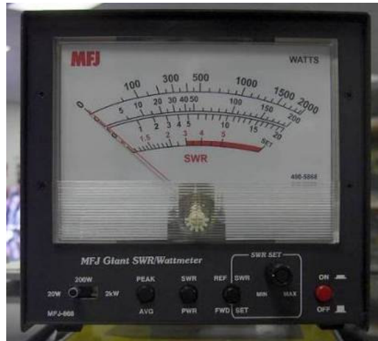
Figure 55 - MFJ's Giant SWR/Wattmeter. Photo by N5IUT
