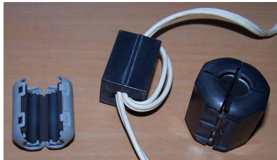
Figure 37 - Three types of Snap-on Chokes. Photo by N5IUT
