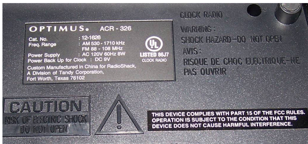
Figure 38 - Part 15 Label from a Clock Radio. Photo by N5IU
