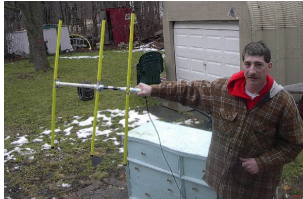
Figure 46 - KA8VIT and a RDF 3 element beam made from a tape measure. Photo by KA8VIT
